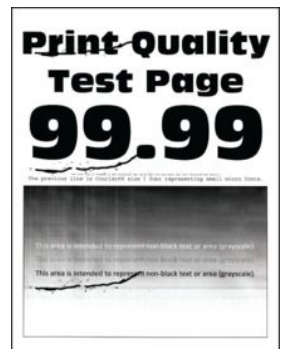
Repeating defects on page 141
