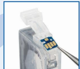
4. With the inlet on the left, click the chip behind the attachment points on the new ink cartridge. First at the top, then the bottom.
